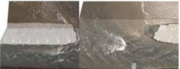
破堤幅  $\approx$  49m (t=78min)
