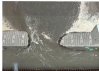
破堤幅  $\approx$  25m (t=64min)
