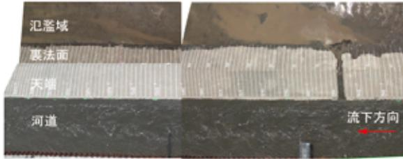
破堤幅≒10m (t=52min)
