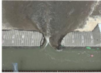
破堤幅  $\approx$  16m (t=39min)
