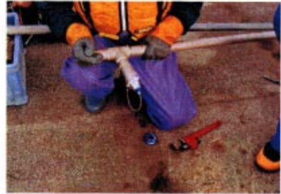
Photo - 2 Device for measuring dynamic hydropressure
